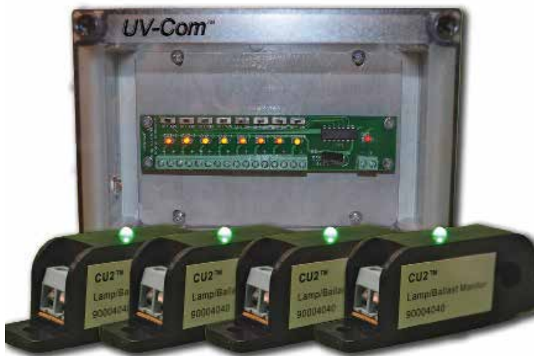
FIGURE 8: Multiple lamp sensors can be fed into a replicator so that one signal is relayed to building management, representing up to eight lamps.
